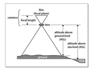
If a camera's focal length is 152 mm, and the plane's altitude Above Ground Level (AGL) is 7 600 m, using the same equation as above, the scale would be:
